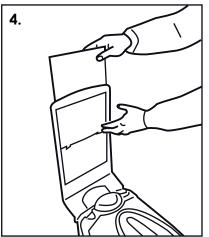
Place the A4 sign behind the clear polycarbonate sheet and slide into the sign carrier so that the lugs locate into the slots along the bottom of the sign carrier.
