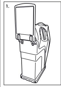
Open the bin door and position the sign carrier at the rear of the bin so that the holes are aligned with the holes in the bin.
