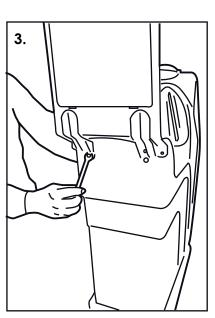
Using a 10mm spanner and allen key tighten the nuts until secure.
