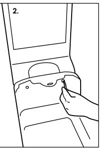
From the inside of the bin, place 4 off screws with washers provided through the holes and fix onto the back of the bin with the washers and nyloc nuts (using your fingers.)
